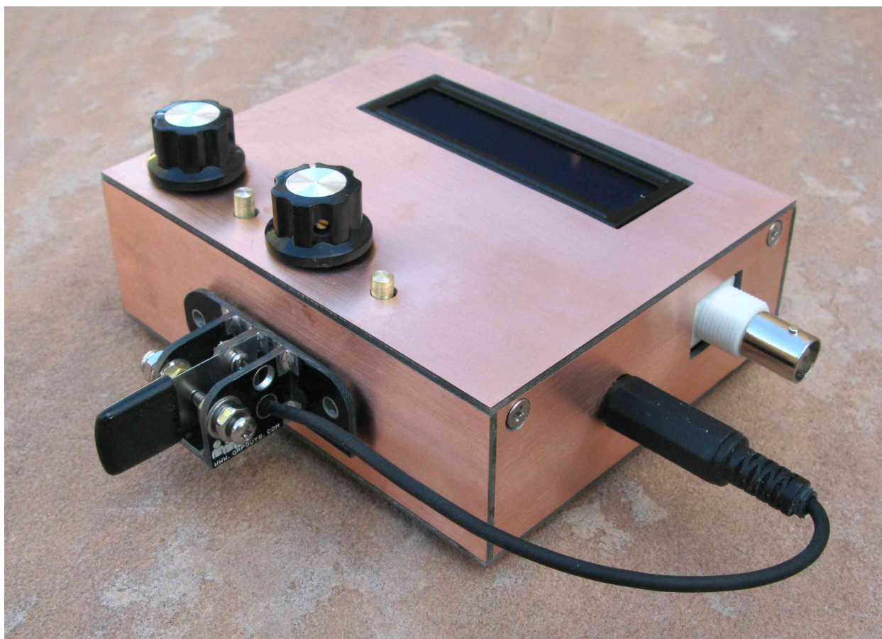
Final fit check before edge radii and painting
